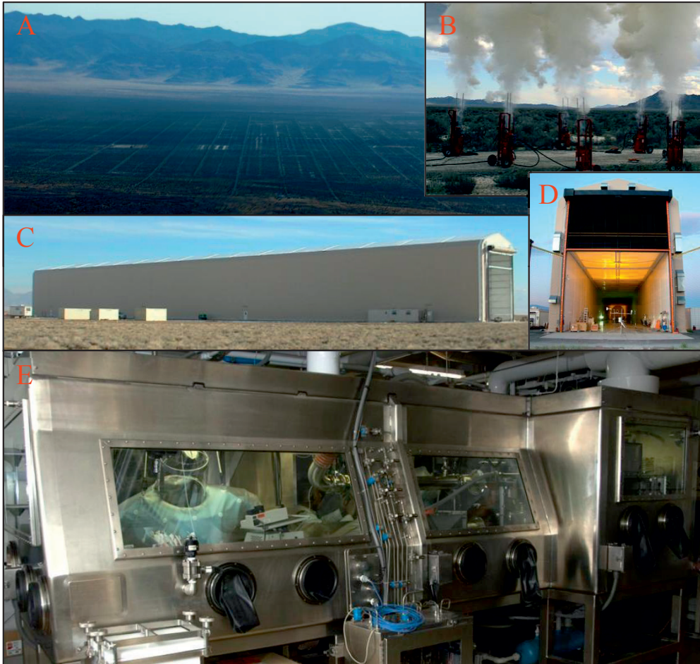
Figure 3. Examples of aerosol test facilities that may be used for T&E of BioDIM systems. Panel A-B: Open-air test ranges. Panel C-D: Ambient breeze tunnels. Panel E: Containment aerosol test chambers. Image credit: Dugway Proving Ground. Printed with permission.
