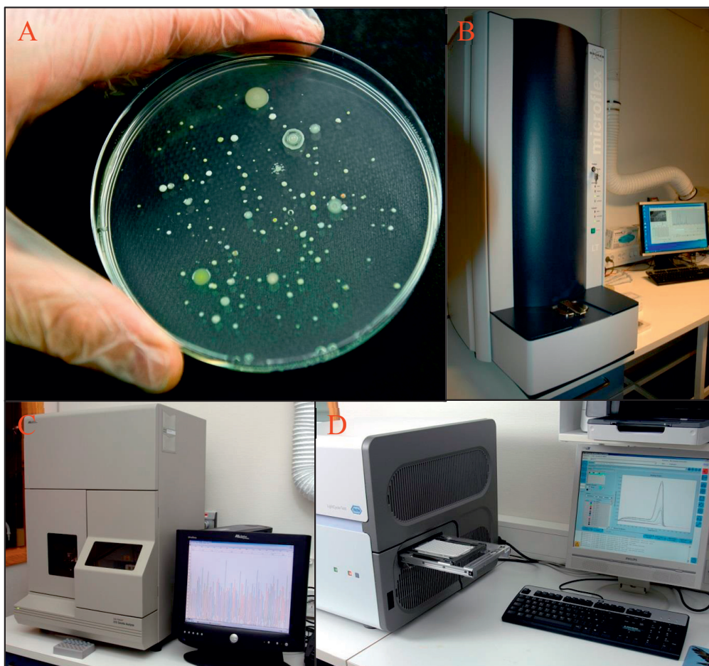
Figure 10. Examples of analysis methods that may be used for quantification and/or identification of airborne bacteria. Panel A: Plate cultivation may be used to quantify airborne bacteria and to obtain bacterial isolate collections (R2A agar plate showing bacterial colonies cultured from a subway station air sample). Panel B: Identification of airborne bacteria may be done using matrix-assisted laser desorption ionization time-of-flight mass spectrometry (MALDI-TOF MS) analysis of bacterial isolates (Microflex LT instrument from Bruker Daltonics, Bremen, Germany). Panel C: Identification of airborne bacteria may be done using Sanger sequencing of 16S rRNA genes from bacterial isolates or clone libraries (ABI 310 Genetic analyzer, Applied Biosystems, Foster City, CA). Panel D: Quantification (qPCR) and identification (e.g. PCR-based identification assays) of airborne bacteria may be done using real-time PCR (LightCycler 480 real-time PCR instrument, Roche Diagnostics, Indianapolis, IN). Image credit: Norwegian Defence Research Establishment.
