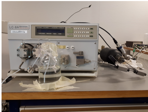
Figure 3.6: The Pump system used in test 1. The accumulator can be observed on the right hand side of the chromatograph.
