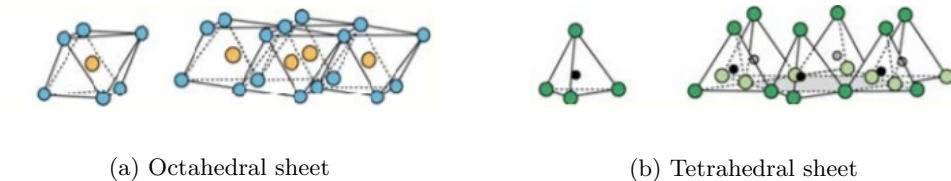
Figure 1.1: Building blocks of clay minerals (Modified from (Eslinger and Pevear, 1988))
