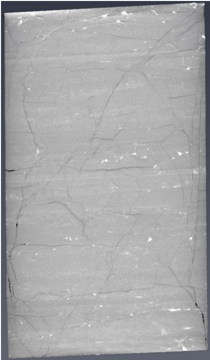
(a) One vertical and one horizontal cross sections of sample 2 after testing.
