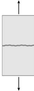
Figure 3: Tensile failure (Modified from Fjær et al. (2008))
