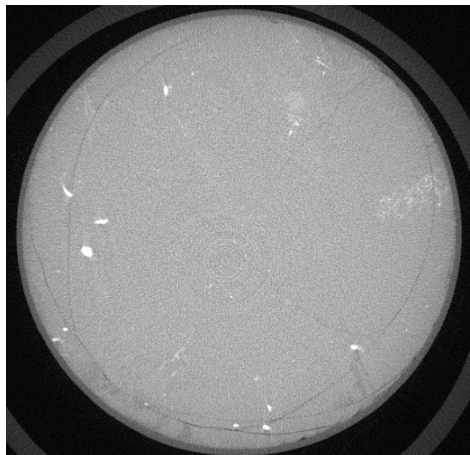
(b) Two horizontal cross section of sample 1 after testing.
