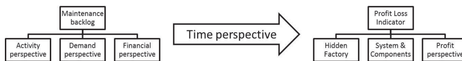
Figure 1 – Measurement of Maintenance backlog as a leading KPI can reduce the value of Profit Loss Indicator as a lagging KPI.
