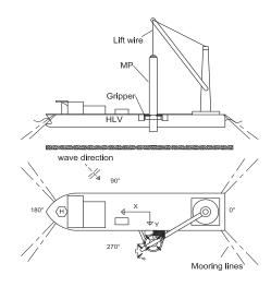
Figure 1: System set-up for the MP lowering operation using a HLV
