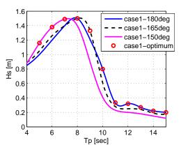
Figure 11: Comparison on allowable sea states for Case 1 with different heading angles
