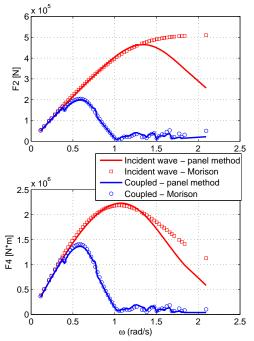
Figure 4: Comparison of excitation force on MP in incident wave and when accounting for shielding effects due to the HLV ( $Dir = 90 \ deg$ , draft = 15 m)
