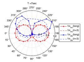
Figure 5: RAOs of fluid X-velocities in incident and disturbed waves with and without wave spreading (T = 7 sec)
