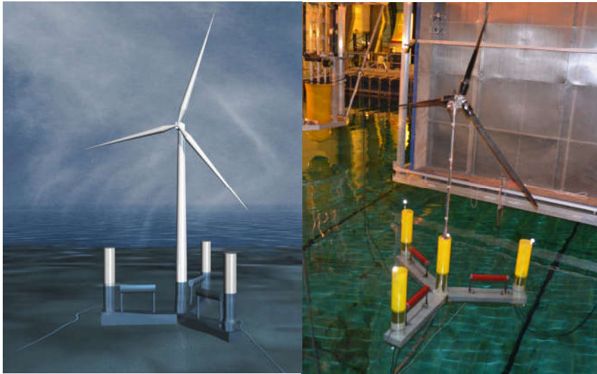
Figure 2. Artistic view of the SFC (Fig. 2a) and the physical model of SFC into the basin (Fig. 2b) (Wind direction is opposite in these two plots)
