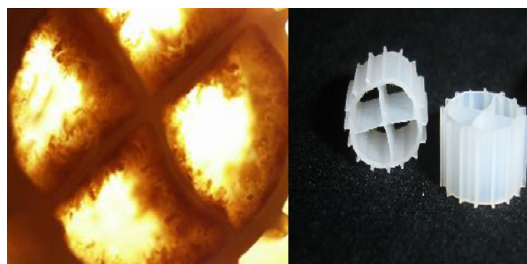
Figure 1.13 – Kaldnes K1 carriers with (left) and without (right) biofilm (Gapes and Keller, 2009)
