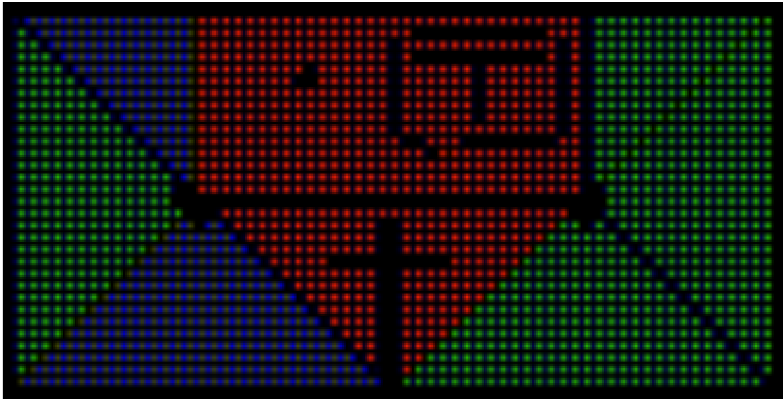
Figure 4.24: Setting the RGB values of 3 out of 4 pixels to 0
