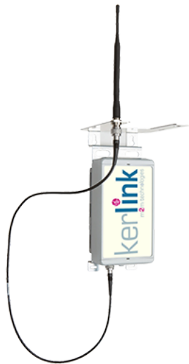
Figure 4.2: A Kerlink gateway used in the CTT project (Source https://www.thethingsnetwork.org/ ).
