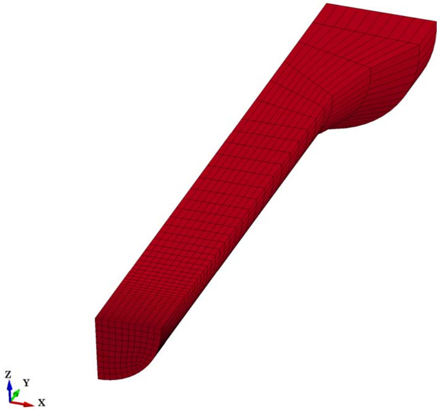
Figure 8: Finite element mesh of the tensile specimen.
