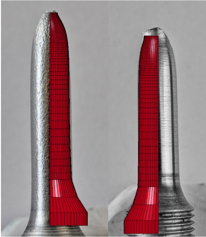
Figure 15: Necking in FEM model and real specimen in 6060-T4 (left) and 6082.25-T6x (right).
