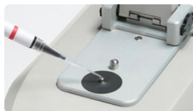
Figure 3.1: NanoDrop® ND-1000 Spectrophotometer . The sample is applied directly to the lower optical surface for measurement of RNA concentration and purity (Modified after [47]).
