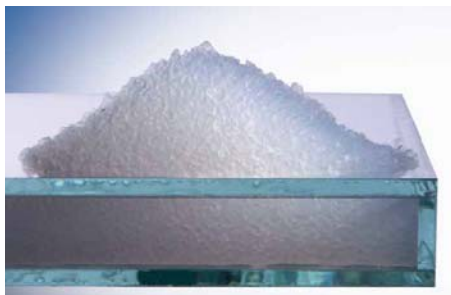
Figure 10. Aerogel granules in glazing (Okalux 2010).
