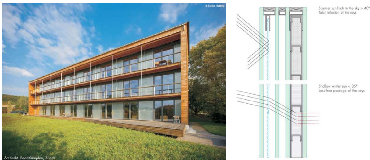
Figure 5. (Left) Building with the GlassX ® crystal translucent wall element incorporating PCMs. (Right) Principal drawing of the GlassX ® crystal PCM window system, see further details in the text (GlassX 2011).
