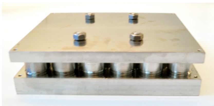
*Figure 2.2. Steel wells utilized for casting of Concordix gels. Each cylinder (6 cylinders are shown between the bottom and top plate) has an interior height=18 cm and diameter=16 cm. The top plate is exerting a press, to ensure equal gel height.*
