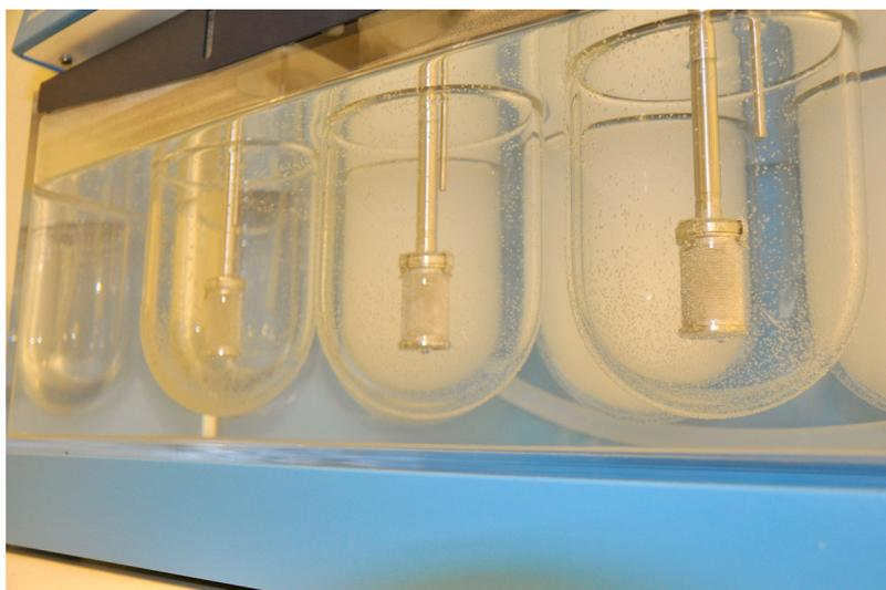
Figure 2.4. The interior of the dissolution unit (SOTAX USP): Three glass beakers are shown (with three additional beakers behind the ones seen), each containing a metal basket, where the gel is placed. Samples are extracted directly from the beaker with a syringe, which is connected to the small metal tube that is seen to the right for the rod holding the basket.
