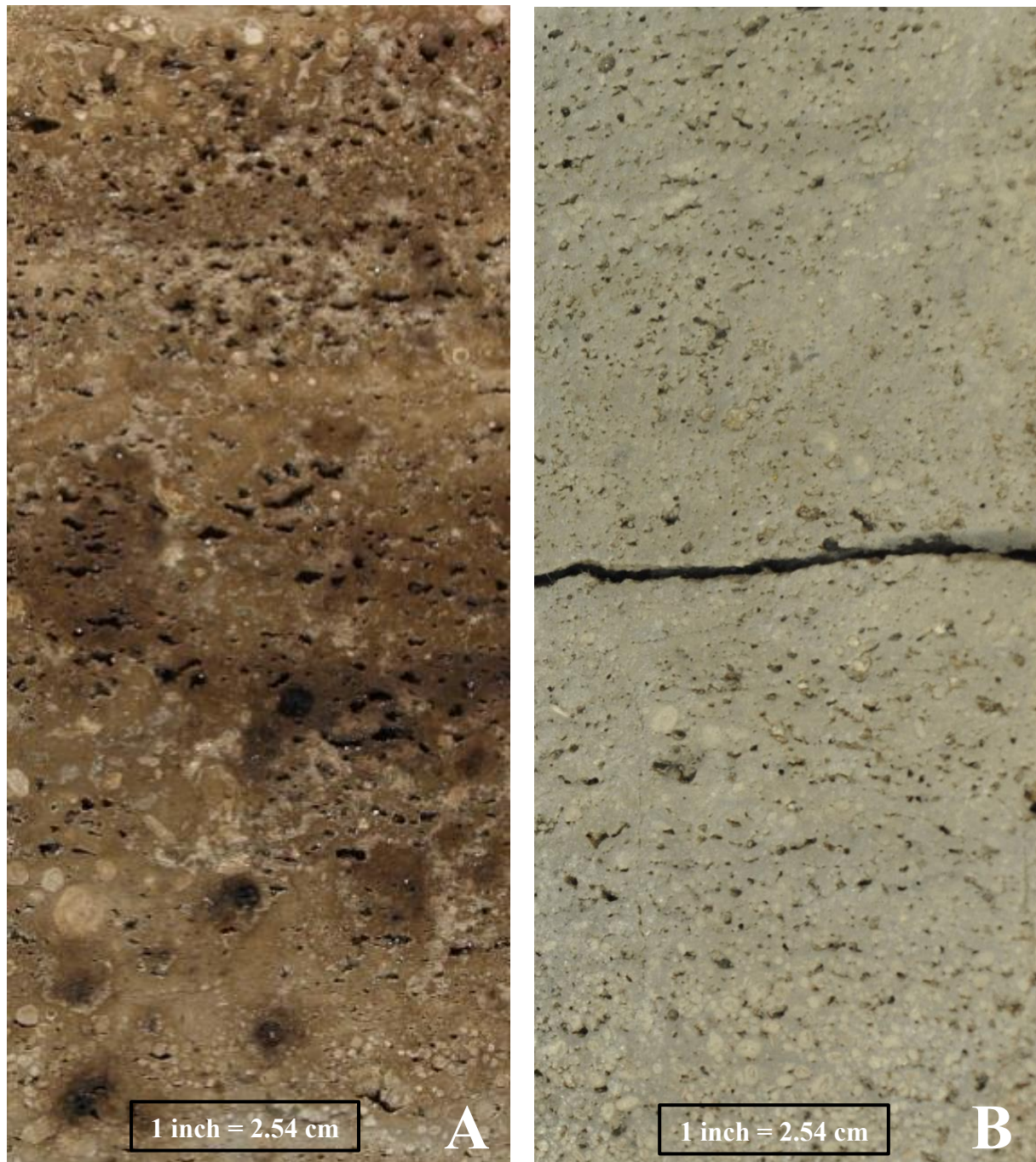
Figure 6.2.6. A). Core slab from Epex Weber 28-9. Depth 1679 m (5507 feet). Brown oolitic-peloid packstone with few skeletal fragments (Facies 9). Enhanced well to very well moldic to vuggy porosity with dark brown oil stains can be observed. B). Core slab from Laura Funke 4. Depth 1597 m. (5241 feet). Different type of a lighter grey, well sorted oolitic to peloid packstone (Facies 9) with a few mud laminae and visible enhanced solution moldic to vuggy porosity.
