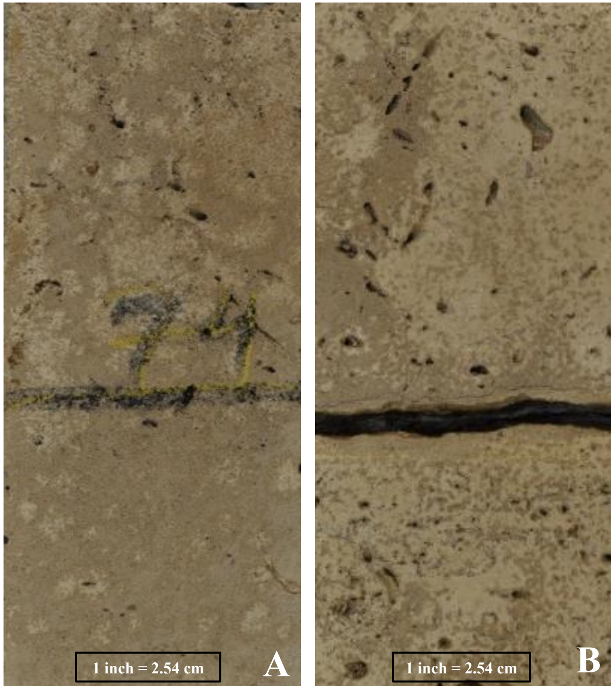
Figure 6.2.9. A). Core slab from Siebert 1. Depth 1699 m (5574 feet). Tan to light brown massive and bioturbated wackestone with a few dissolved skeletal fragments. B). Core slab from Donald Peterson 3-27. Depth 1689 m (5542 feet). Tan to light brown massive and bioturbated wackestone with a few dissolved skeletal fragments.
