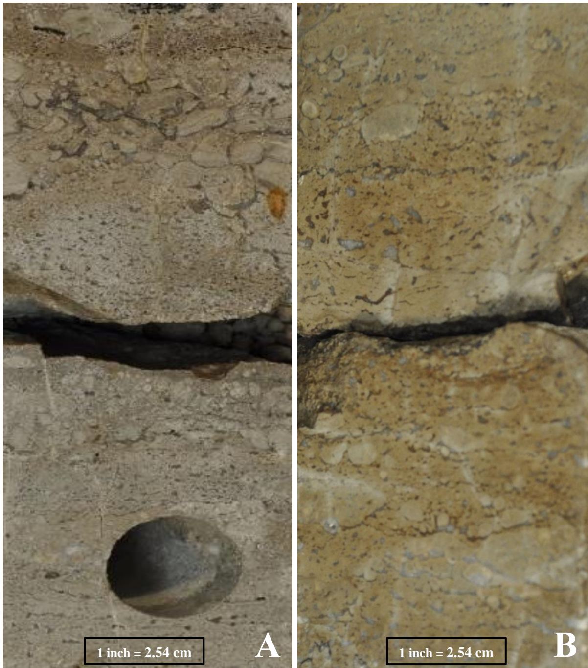
Figure 6.2.1. A). Core slab from Siebert 1. Depth 1681 m (5514 feet). Light grey to brown intraclastic/peloid mixture. Grades into a thin bed with big rounded to angular grains with sharp contacts, indicating some sort of event of erosion and transport of reworked sediments. B). Core slab from Laura Funke 4. Depth 1623 m (5326 feet). Light tan intraclastic packstone with big pieces of lime mud intraclasts, peloid grains within a very poorly sorted and floating muddy texture.
