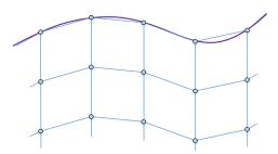
Fig. 3 Distortion due to boundary geometry
