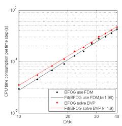
Fig. 26 CPU time consumption per time step by different methods to achieve  $\partial \varphi / \partial t$
