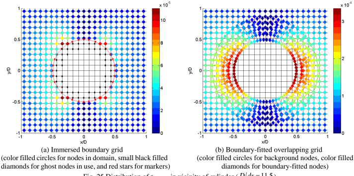
Fig. 25 Distribution of  $e_{\varphi,GS,rel}$  in vicinity of cylinder (D/dx = 11.5)
