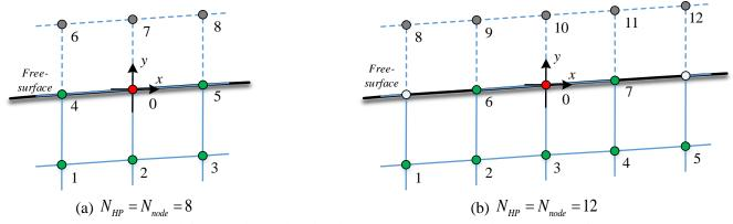
Fig. 32 Cells used for velocity estimation in the BFOG method with one layer of ghost nodes
