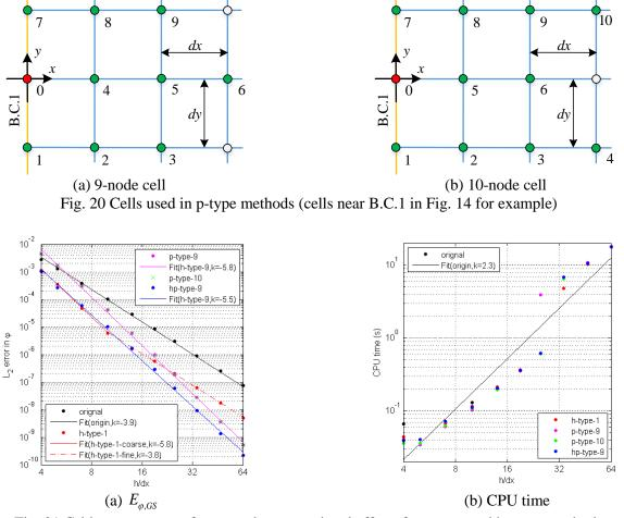
Fig. 21 Grid convergence of error and computational efforts for p-type and hp-type methods
