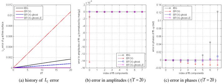
Fig. 34 Error in potential on the free-surface ( $\lambda/dx = 32$ )
