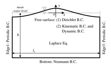
Fig. 28 Computational domain and boundary conditions for a nonlinear wave tank with periodic edges
