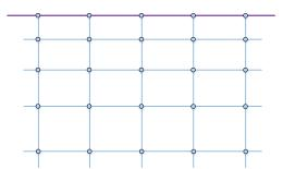
Fig. 2 Refinement in one direction (stretching)
