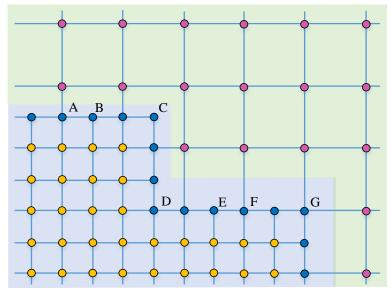
Fig. 11 Typical Quadtree grid
