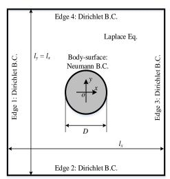
Fig. 23 Computational domain and boundary conditions for potential flow around a submerged cylinder
