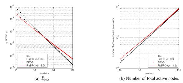
Fig. 29 Grid convergence of  $E_{\alpha,GS}$  and total number of active nodes for numerical wave-tank
