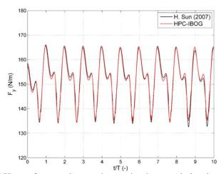
Fig. 37 Heave force acting on the semi-submerged circular cylinder
