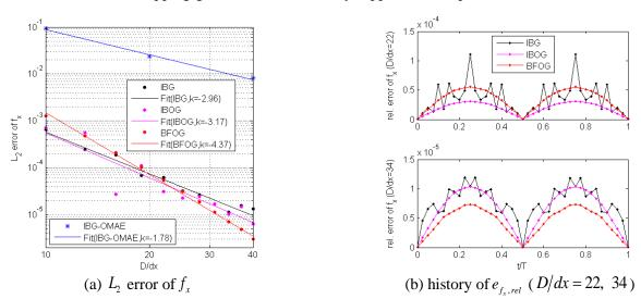
Fig. 27 Error in  $f_x$  for different grid methods
