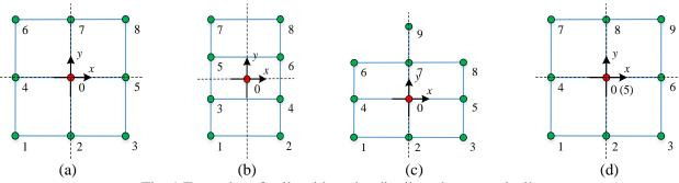
Fig. 1 Examples of cells with nodes distributed symmetrically
