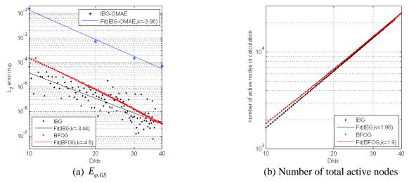
Fig. 24 Grid convergence of  $E_{\varphi,GS}$  and number of total active nodes for submerged cylinder example
