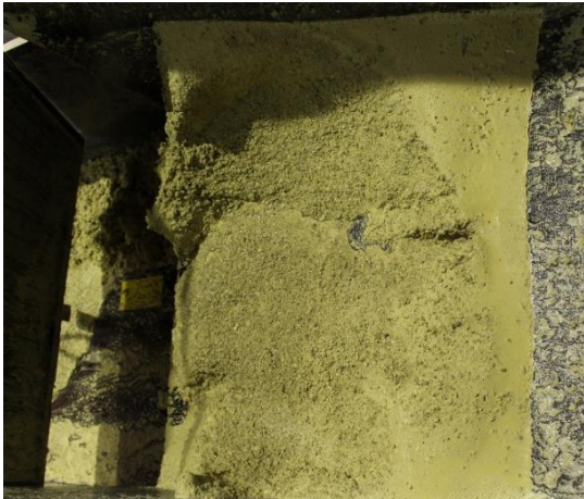
Figure 3-6 Material remained in the box with the test using 80 kg of fine material and 20 kg of material
