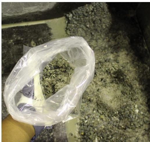
Figure 3-11 Samples collected to measure water content of the material left inside the box after test
