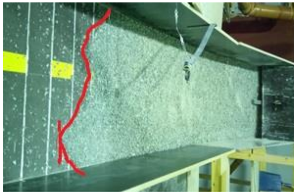
Figure 4-10 Indication of the point for runout length measurement for the debris slide
