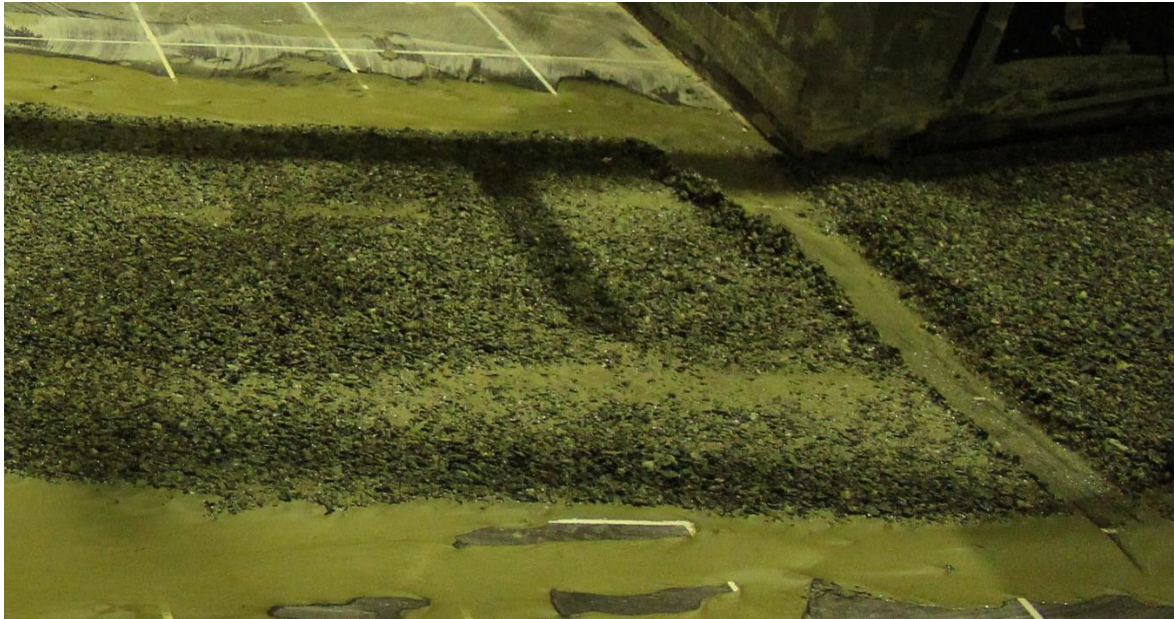
Figure 5-16 Inverse grading of the deposition pattern for test 24 (40+12 combination)
