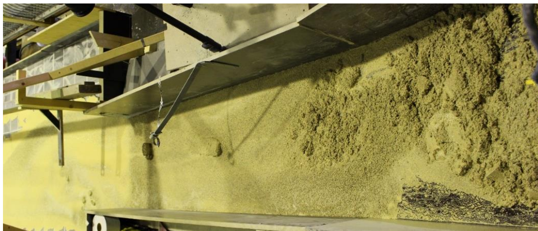
Figure 3-8 Frozen material as seen during the flow with the fine material
