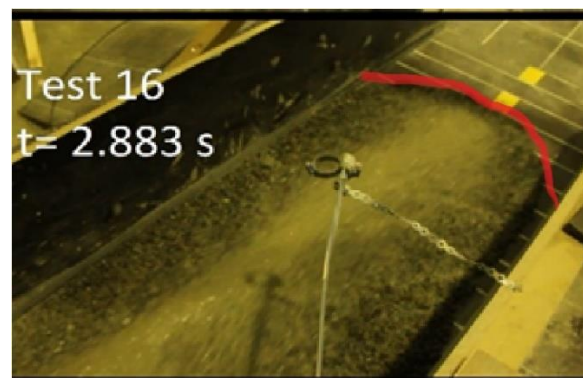
Figure 5-2 Debris flow front for test 16 at time 2.883 s
