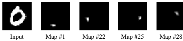
Figure 5.9: Visualizations produced using a deconvolutional network for the visualization input image in a . A selection of four different feature maps from the pool layer is displayed.
