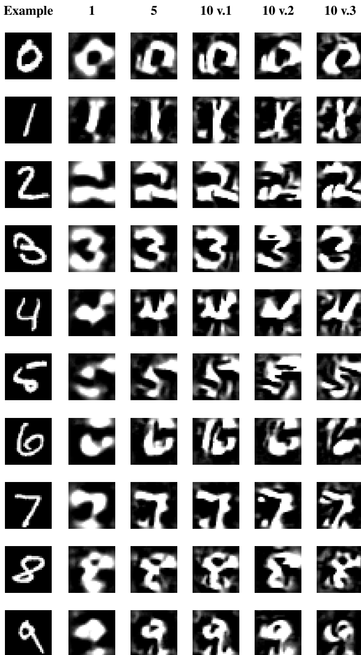
Figure 5.10: Deep visualization of the output layer for all 10 output classes of the MNIST network. An example image from each class is shown in the first column. Column 2-4 shows samples collected at certain stages of training. The two training epochs consisted of ten evenly distributed stages. The last three columns show the variations acquired from multiple deep visualization from the same unit.
