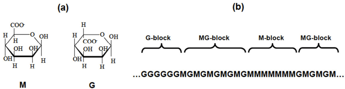
Figure 1.1: Alginate chemical structure. (a) Illustration of the Haworth formulas of the two monomers. M = \beta -D-mannuronic acid and G = \alpha -L-guluronic acid. (b) Block composition in alginates (excerpt directly reproduced from (Mørch, 2008)).
