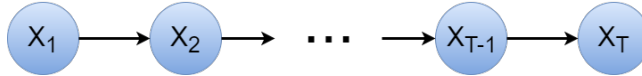
Figure 3.1: Illustration of a first order Markov chain. The arrows represent the dependencies between the nodes.
