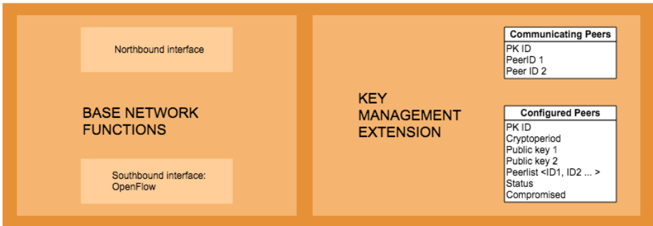
Figure 4.2: Controller illustrated with its key management extensions which shows two tables, one displaying the peers communicating, while the other contains all configured peers.
