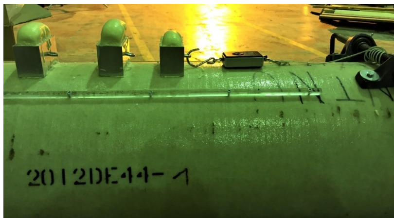
Figure 10: Setup of the adhesion test rig
