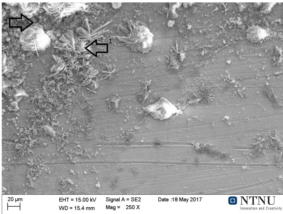
Figure 4.37: SEM Image of X65 carbon steel from galvanic crevice corrosion with cathodic protection at 10°C run for 96 hours. Image is taken before chemical cleaning and is taken of the area which was indicated in black on figure 4.36. EDS analysis is performed at the points indicated in black
