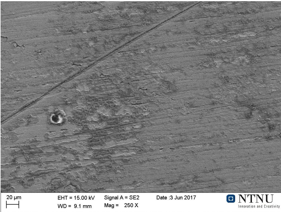
Figure 4.33: SEM Image of X65 carbon steel from galvanic crevice corrosion at 10°C run for 120 hours with cathodic protection. Image is taken after chemical cleaning and is taken of the top of the sample
