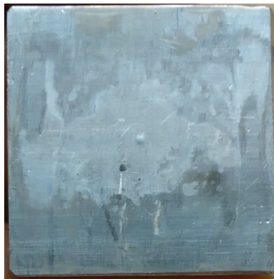
Figure 4.19: Photograph of 6005 surface after chemical cleaning
