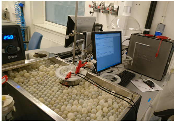
Figure 3.6: Picture of the setup on the lab. The cell is submerged in an water bath holding 25°C. The reference electrode is connected through a salt bridge. One of the potentiostats are pictured with a plot of the ongoing recordings
