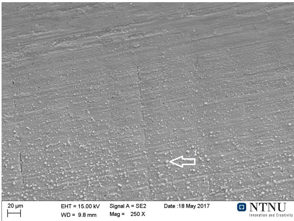
Figure 4.35: SEM Image of 6005 aluminum from galvanic crevice corrosion without cathodic protection at 10°C run for 96 hours. Image is taken before chemical cleaning and is taken at the bottom of the sample. EDS analysis is performed on the particle marked in white
