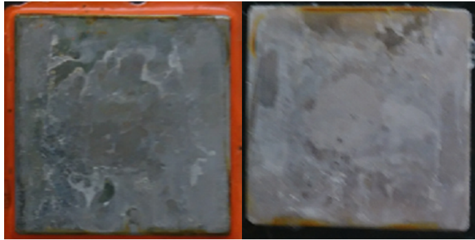
(a) X 65 steel from galvanic crevice corrosion testing without cathodic protection. Image is taken before chemical cleaning
