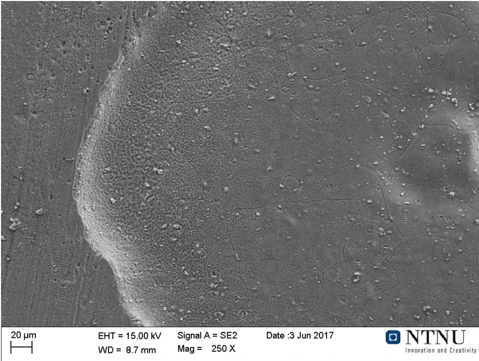
Figure 6.16: SEM Image of 6005 aluminum from galvanic crevice corrosion at 10^\circ run for 120 hours. Image is taken after chemical cleaning and is taken in the middle
