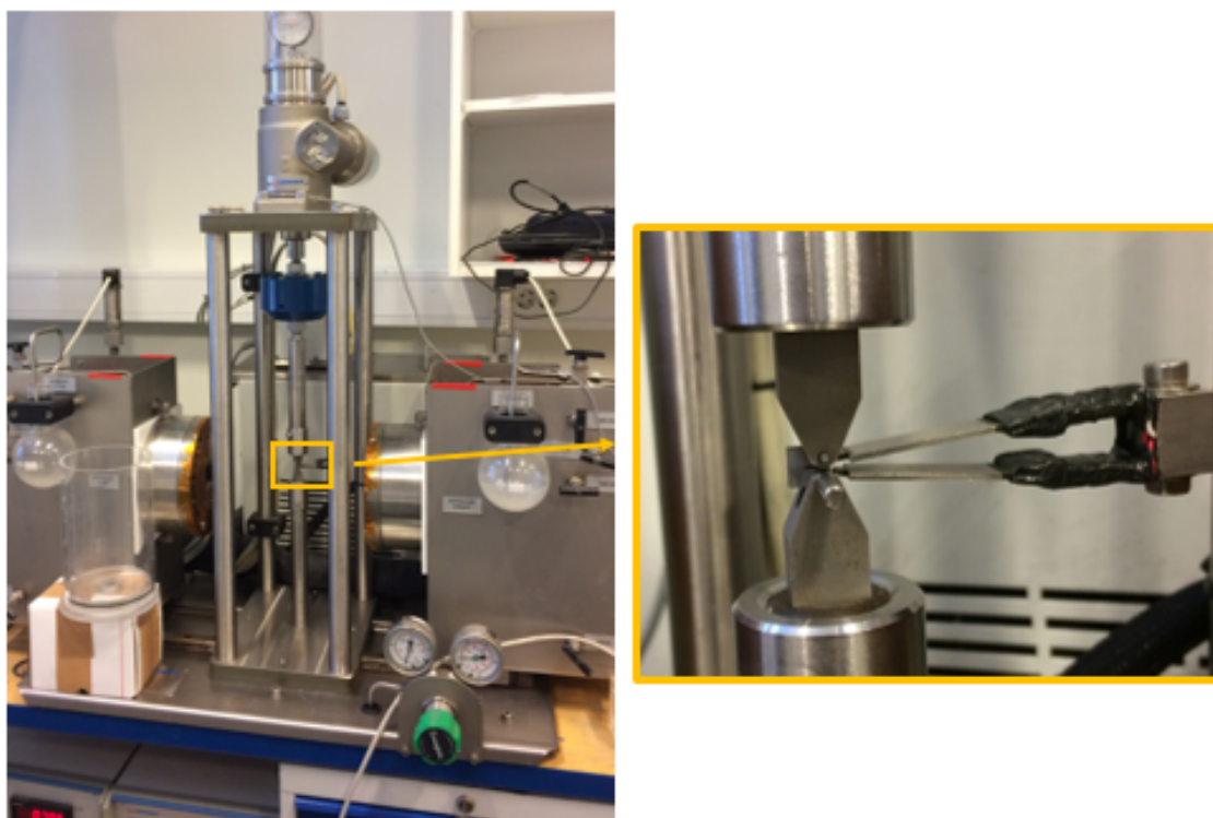
Figure 3.5: Cormet slow strain rate test rig, test setup in air.
