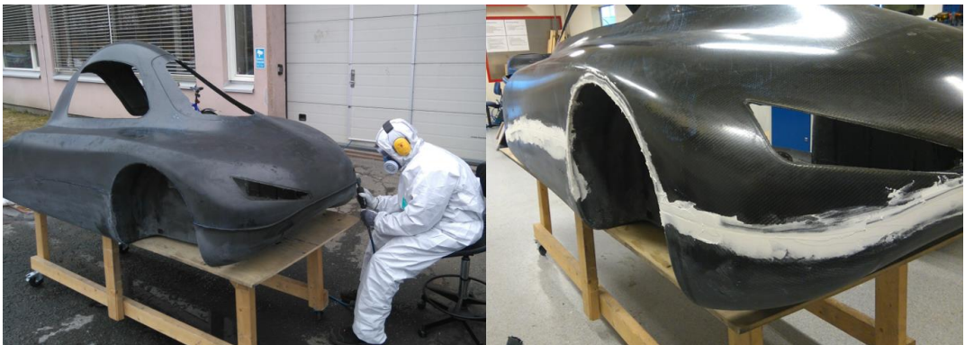
Figure 40:Grinding flanges off and plastering joint line
