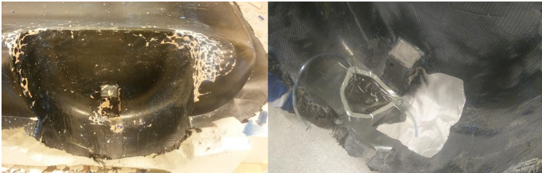
Figure 37: Left: Remains of mould on body. Right: Applying resin to dry spot
