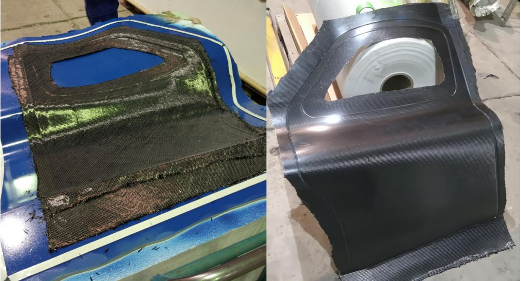
Figure 23: Left: Carbon fibre lay-up. Right: Door out of mould
