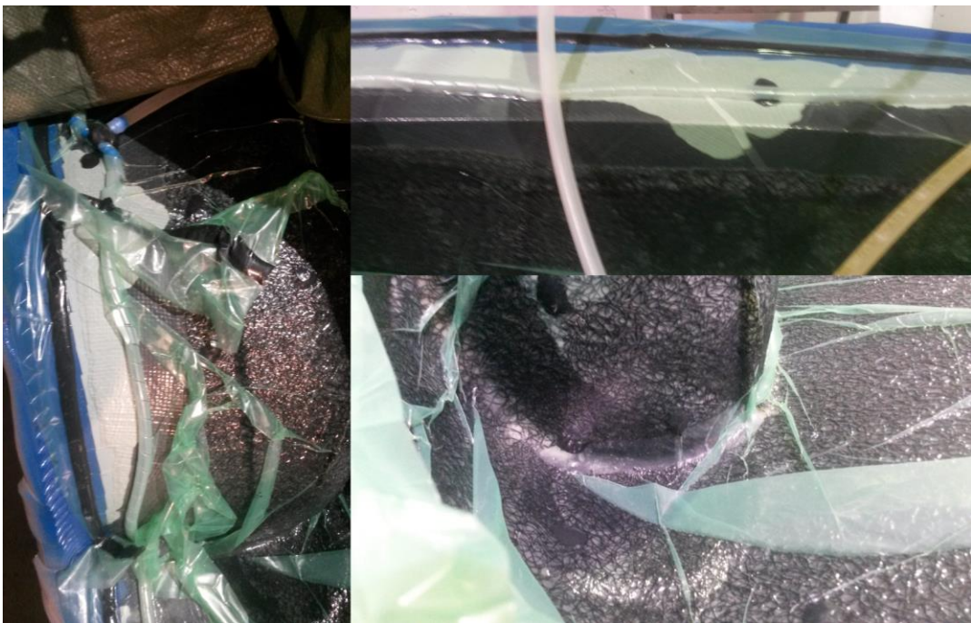
Figure 36: Left: Dry spot on wheel arch. Top right: Dry spot on right side. Bottom right: Accumulation of resin in the edge
