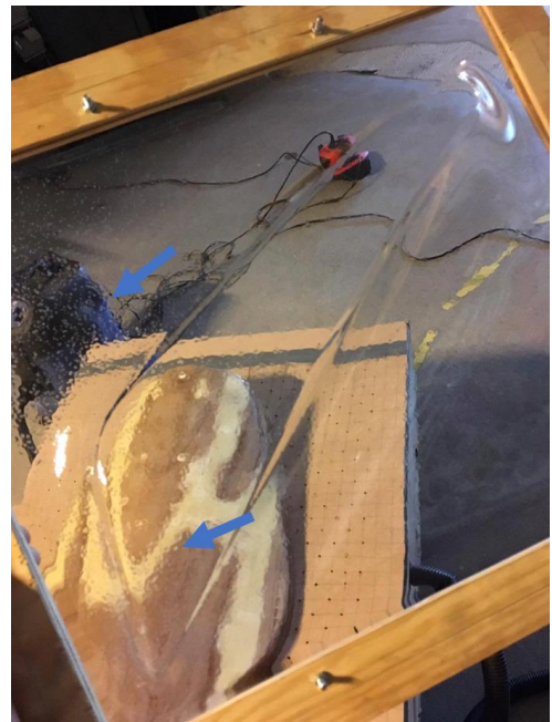
Figure 87: Bubbles in the Lexan
