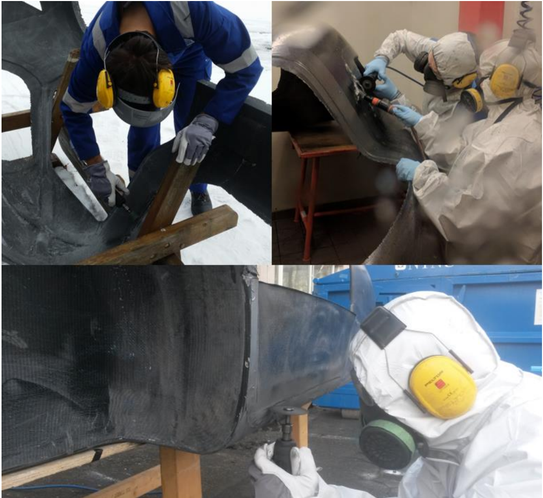
Figure 38: Grinding excess resin and trimming body
