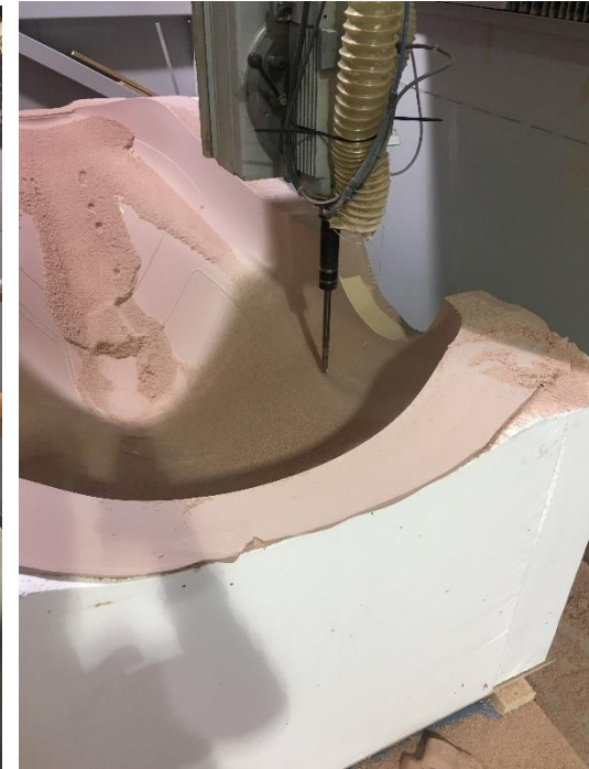
Figure 20: Production of moulds at Eker design. Epoxy paste is used to give the moulds a hard surface
