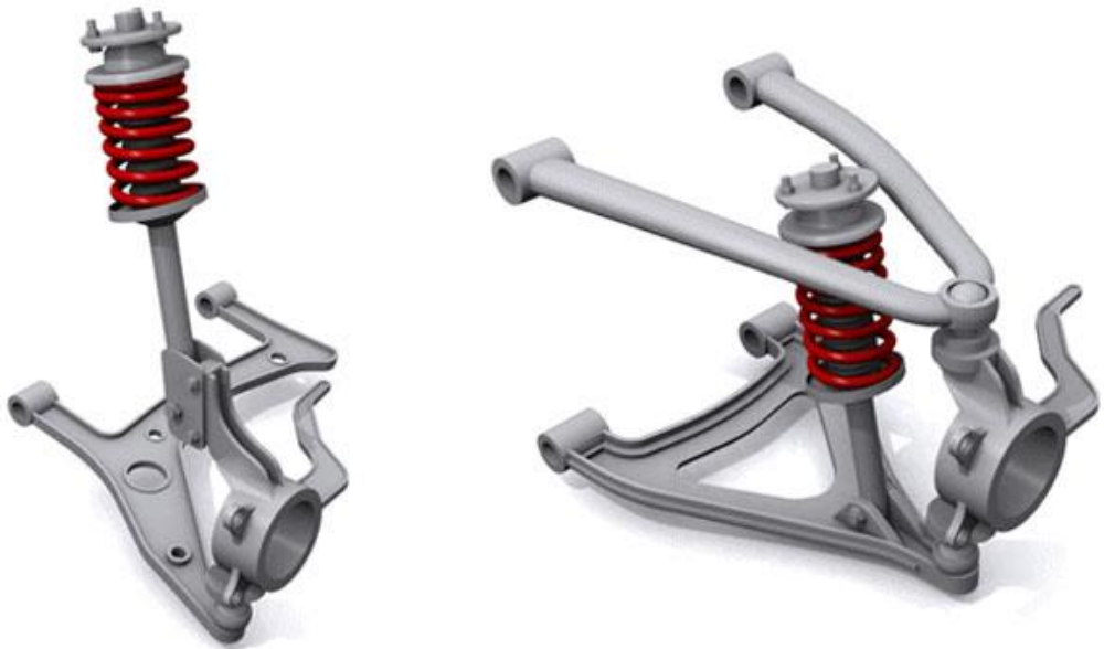
Figure 137: MacPherson strut (left) and double wishbone suspension (right)
