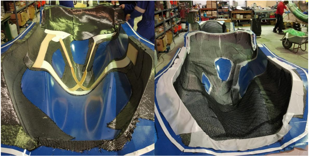
Figure 26: Left: Core material. Right: Peel ply and flow mesh
