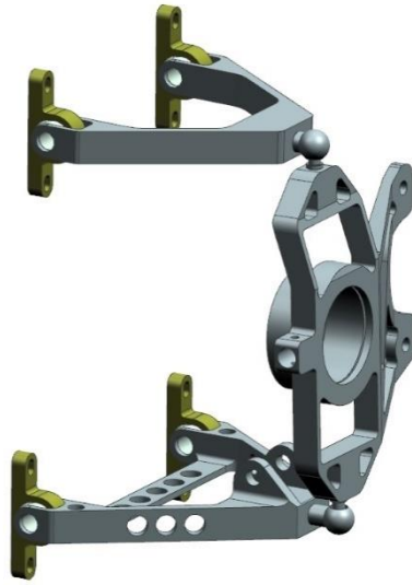
Figure 66: Final design of the wishbones and the steering knuckle
