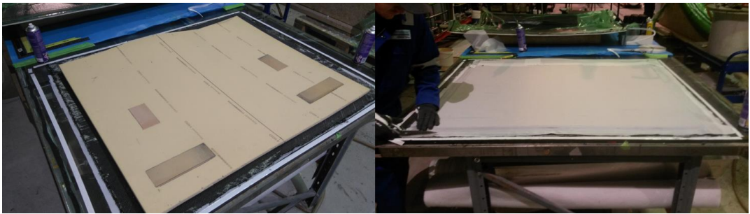
Figure 29: Left: Inserts in core material. Right: Covered with peel ply
