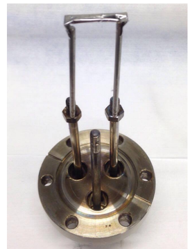
Figure 3.4: Photo of a home-made Dy evaporator. Taken from Ref. 19.
