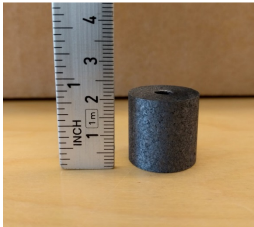
Figure 2.2-1: The graphite piece used as anode.
