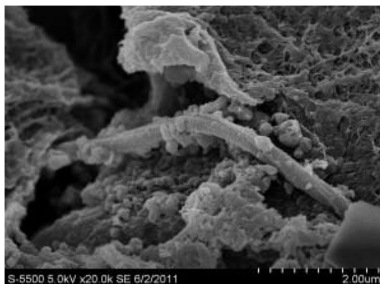
Figure 3.30 Collagen fibers interacting with both mineral composites, and the alginate matrix. The collagen was observed in sample 4a, which is given ALP and differentiation medium. Magnification: 20 k.
