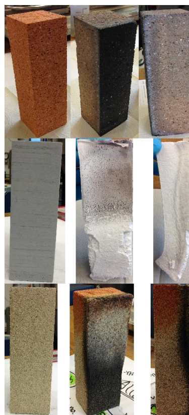
Figure 2. From top to bottom: Moler SUPRA, SUPER-1100 E calcium silicate, and V-1100 (475) vermiculite. The left picture of each material shows the pristine material, while the others show the material after the sodium vapour test. The middle pictures show the side of the bar facing the carbon crucible.
