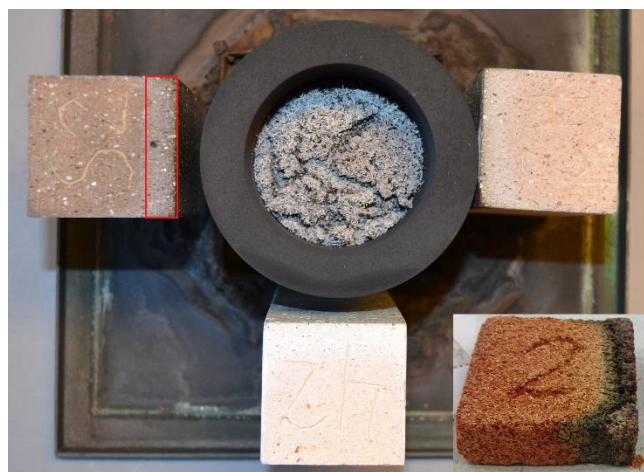
Figure 1. Setup for the sodium vapour test with the materials facing the carbon crucible holding the reactants. The red square indicates the part cut out and used for X-ray diffraction analysis. The lower right picture shows a horizontal cross section cut from the sodium exposed vermiculite material.
