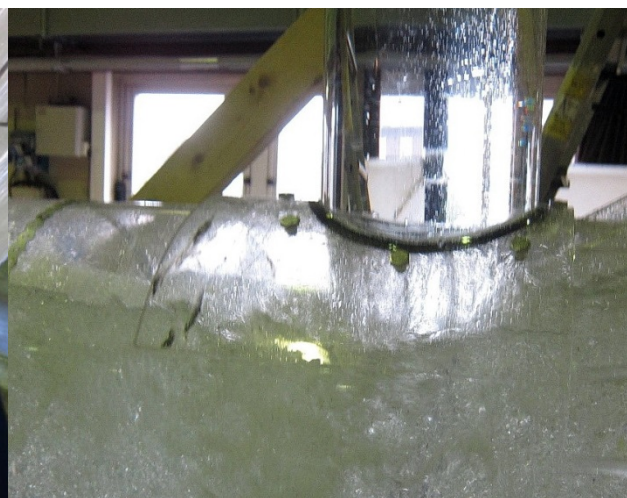
Figure 32- Air accumulation in tunnel with 90^{\circ} shaft
