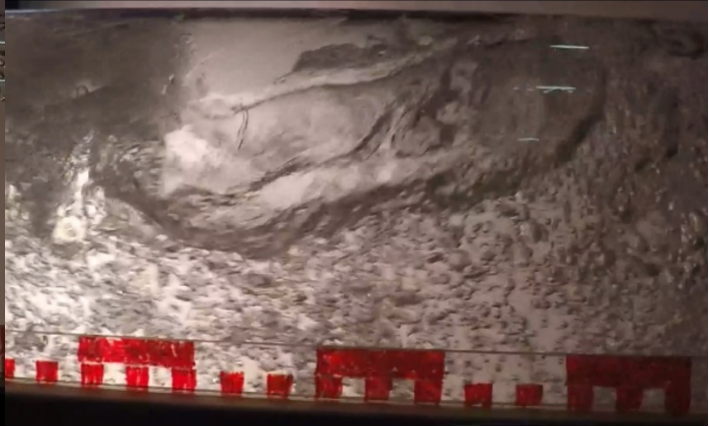
Figure 22-Type 4 regime, 45 o , 1.3% air, 30l/s, bubble is closing
