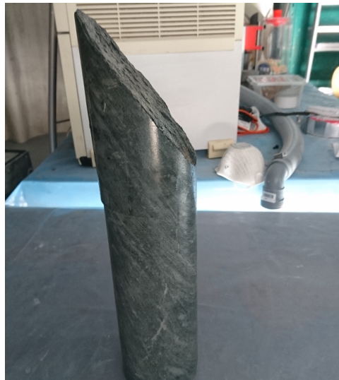
Figure 13: A typical inclined surface (this is the rock part from one core)
