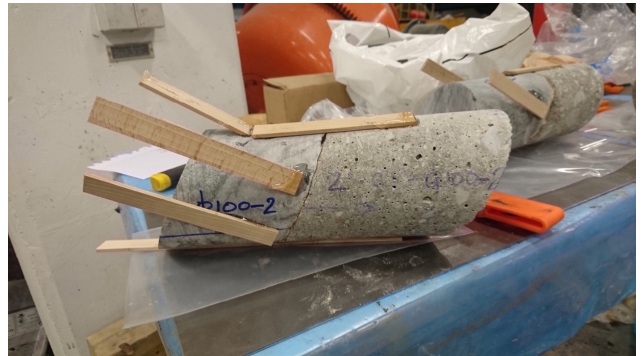
Figure 79: The rock and concrete were glued together to keep them mated when casting the samples
