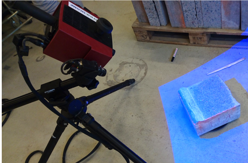
Figure 19: Scanning of surface with ATOS 5MP. (this is a sample from another test series that were conducted at LTU in the same period)
