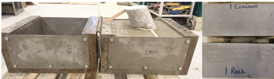
Figure 16: A sample during encapsulation of the rock part, and a sample that is ready for testing
