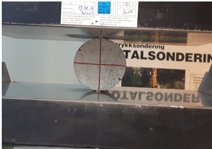
Figure 36: Test apparatus and set up for splitting tests
