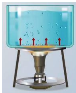
Figure 10 – Maximum heat flux, more bubbles are generated and contact area decreases [26]
