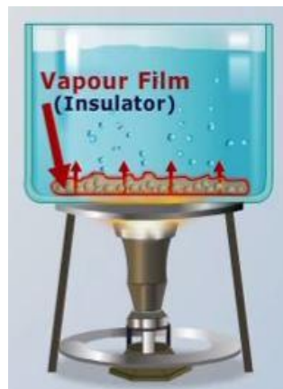
Figure 11 – Transition boiling regime, continuous vapor film is formed and further decrease of the contact area [26]
