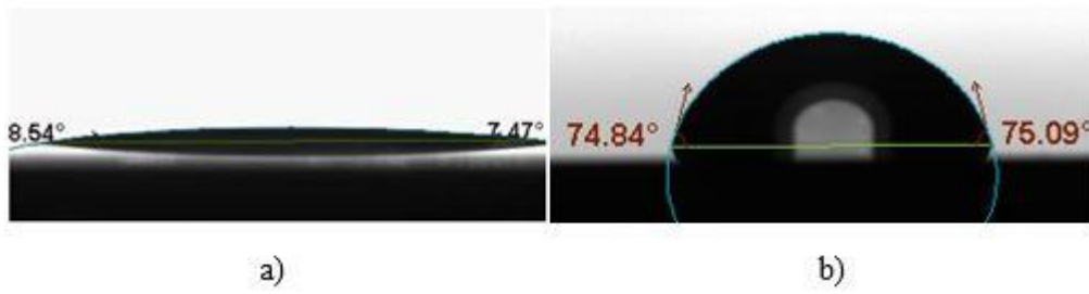
Figure 77 – a) water contact angle on Si nanowires Diameter 800 nm Pitch 2 \mu\text{m} Height 2 \mu\text{m} b) water contact angle on plain polished silicon
