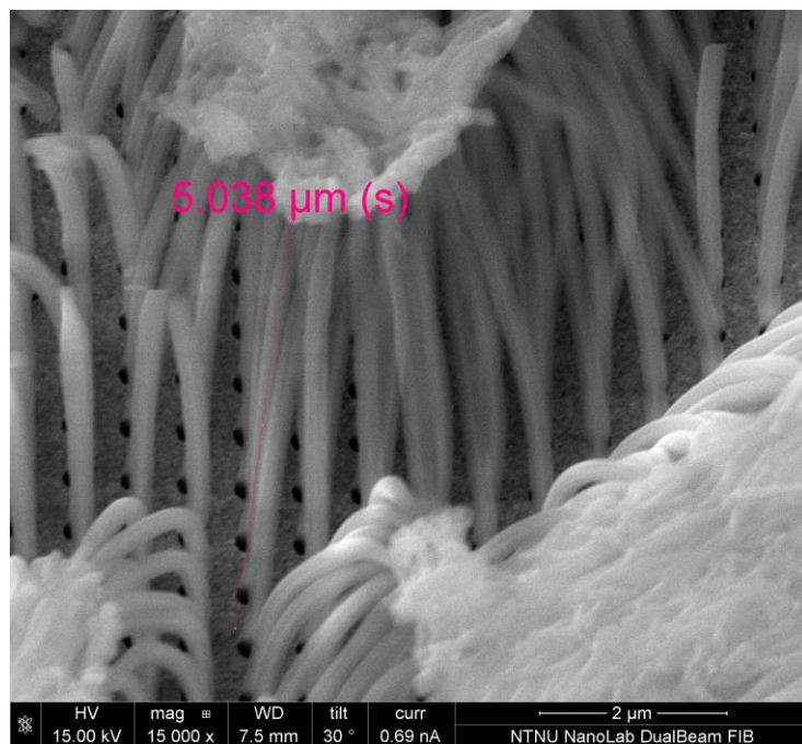
Figure 70 - Banded Si nanowires after etching Diameter 200 nm Pitch 625 nm, tilted 30°
