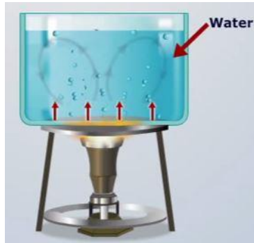
Figure 9 - Nucleate boiling regime, vapor bubbles starts to be generated [26]
