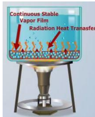
Figure 12 – Film boiling regime, stable vapor film is generated and a significant loss of heat transfer is present [26]
