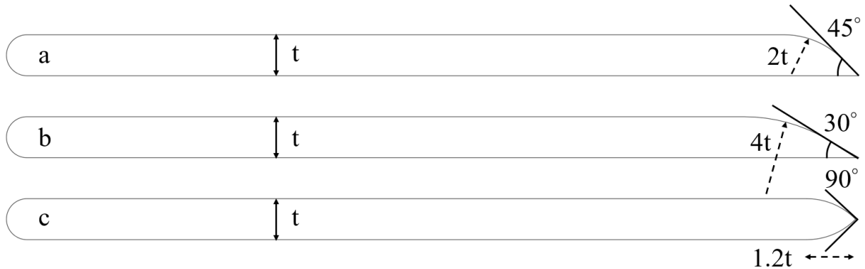
Figure 3.5: Trailing edge designs with constant thickness hydrofoils.
