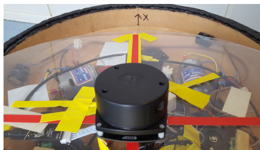
Figure C.2: Lid placement and LIDAR placement, courtesy of Ueland (2016)
