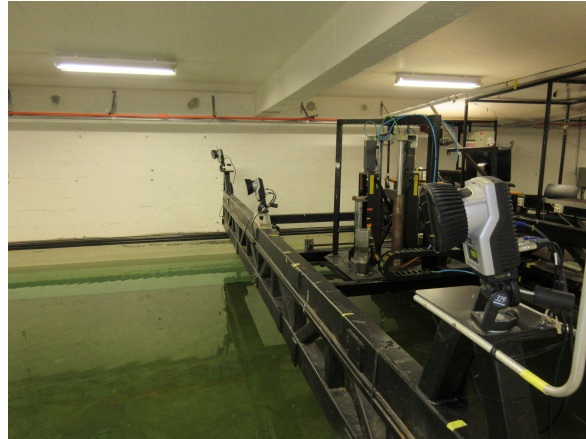
Figure 4.5: The infrared cameras utilized by the Qualisys system
