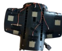
Figure 6-4 Sensor placement in Seat
