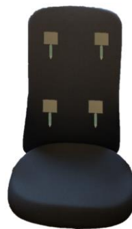
Figure 5-7b Sensor Placement in Backrest
