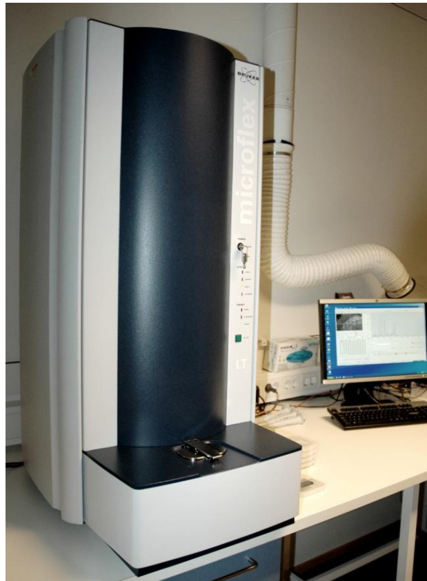
Figure 2.5: MicroFlex MALDI-TOF MS instrument (Bruker Daltonics Inc., Germany) (picture by FFI)
