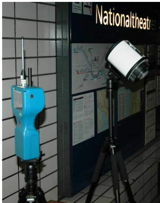
Figure 2.2: Aerotrak 8220 particle counter (left), SASS3100 filter sampler (right) (Picture by FFI)
