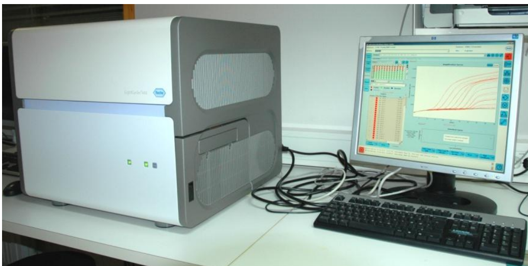
Figure 2.4: LightCycler 480 PCR machine (left) and LightCycler Computer Program (right) (Roche Diagnostics Corp., IN, USA) (Picture by FFI)
