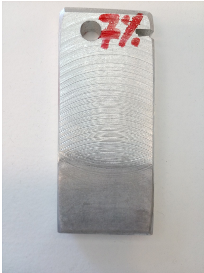
Figure 4.35: Results of store bought vinegar, a 7% etchant solution
