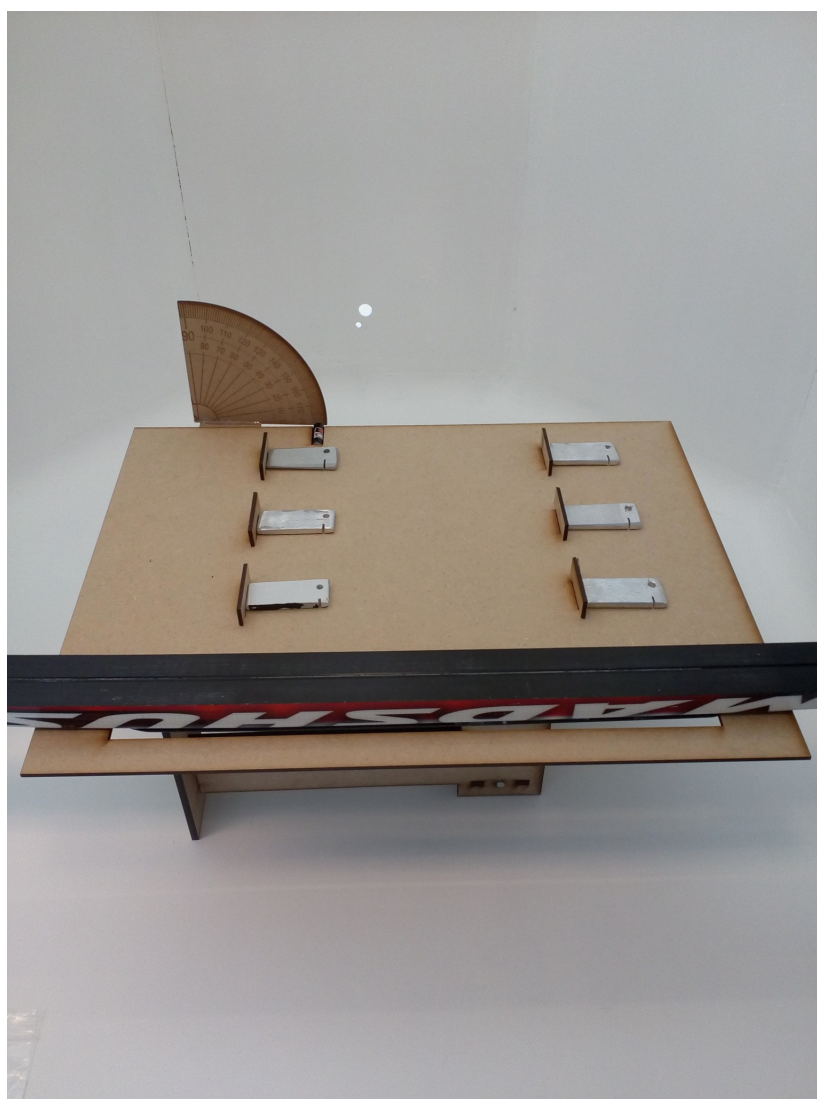
Figure 5.44: Set up for testing roll-off angle of test samples
