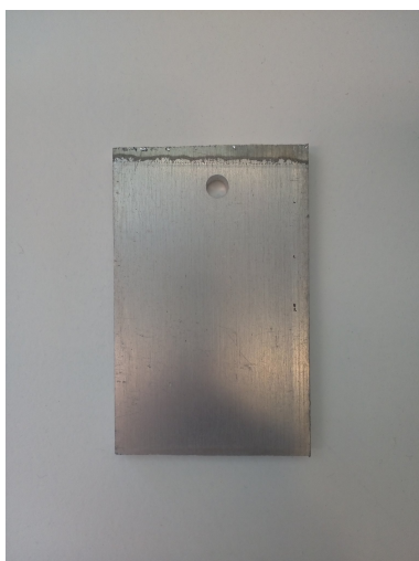
Figure 4.30: Big aluminum plate. Above the hole one can see where the acid surface has stopped reacting with the metal
