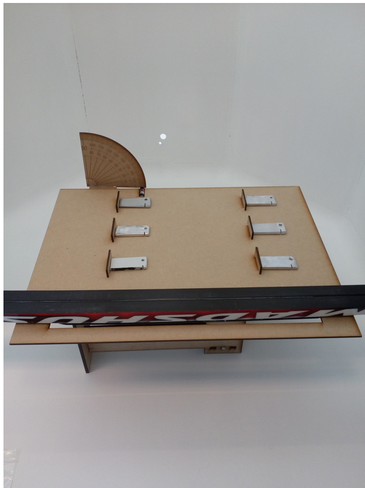
Figure 7.7: The final prototype with both test samples and cross country ski mounted
