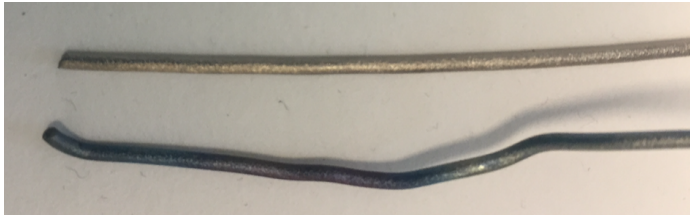
Figure 7.1: Unused titanium on top, anodized blue titanium on bottom
