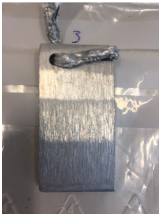
Figure 4.18: Aluminum foil still same color after anodizing
