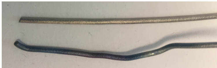
Figure 4.32: Unused titanium on top, anodized blue titanium on bottom
