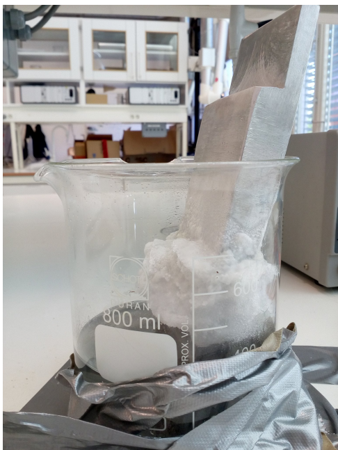
Figure 7.3: Cathode after developing crystal structure on the surface
