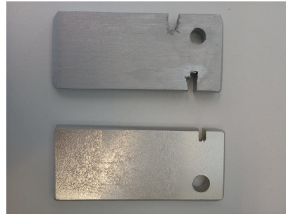
Figure 7.2: Added cuts to increase connection between titanium and aluminum sample
