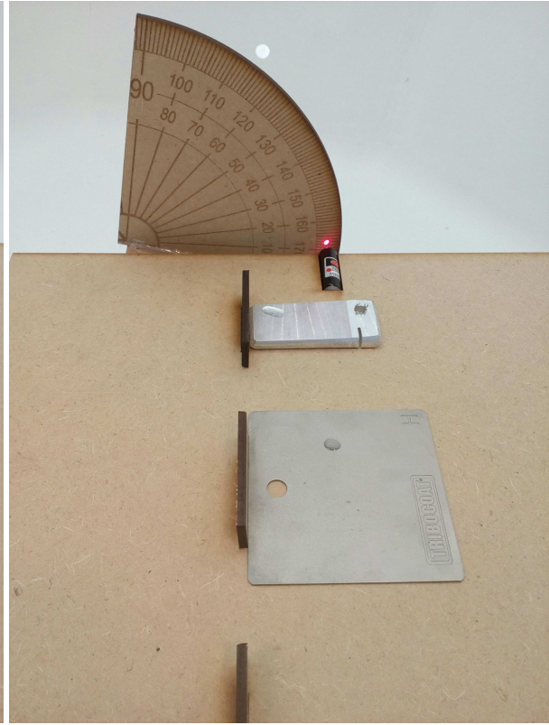
Figure 5.42: Laser diode measuring angle when water droplet starts gliding on the aluminum surface
