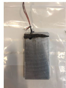
Figure 4.16: Black aluminum wire, showing anodizing has failed
