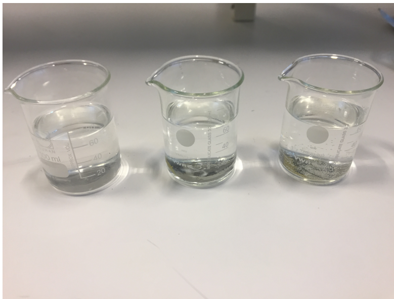
Figure 4.33: Overview of the three solutions used. Acetic ratio from the left is 1:1, middle 1:20, right 1:8
