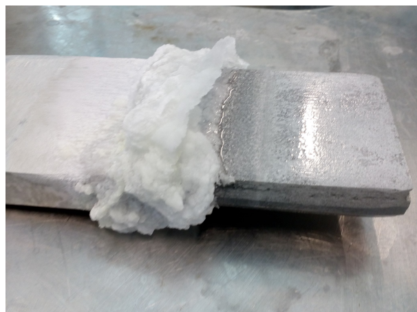
Figure 7.4: Cathode showing clear signs of dissolving because of acid
