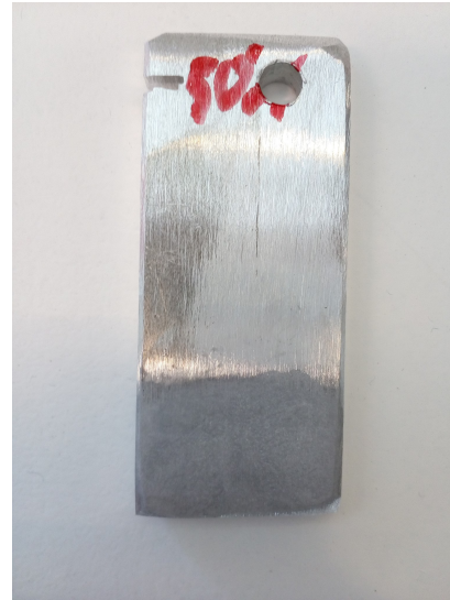
Figure 4.36: Results of acetic acid mixed with water at a 1:20 ratio.
