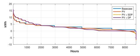
Figure C.2: Duration curves of  $P_{grid}$  for 2016 for load 3 with PV under the time based UT.
