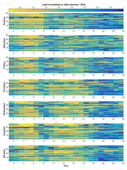
Figure D.8: Normalised load for load 2 in 2016, sorted by days.
