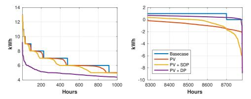
Figure C.6: Duration curves of  $P_{grid}$  for 2016 for load 3 with PV under the power based UT, zoomed in for maximum 1 000 hours and minimum 500 hours.
