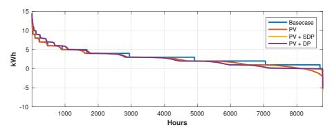
Figure C.1: Duration curves of  $P_{grid}$  for 2016 for load 3 with PV under the energy based UT.
