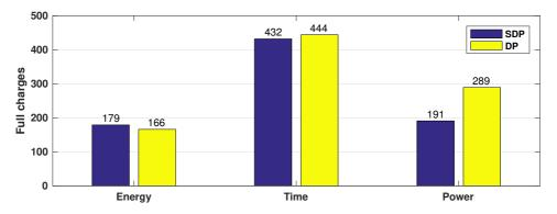
Figure 5.22: Total normalised battery usage counted in number of total recharges under standard settings without PV.
