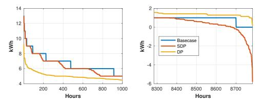
**Figure 5.32:** Duration curves of  $P_{grid}$  for 2016 for load 3 without PV under the power based UT. Maximum 1000 values and minimum 500 values.
