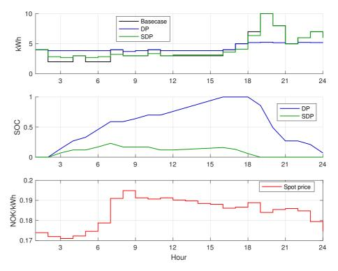
**Figure 5.12:** Friday the 12th of February 2016, standard settings without PV under the power based UT. Upper plot shows  $P_{grid}$  for the basecase, DP and SDP. Middle plot shows the SOC of the battery. Lower plot shows spot price.
