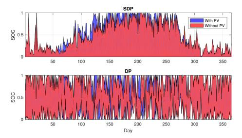
**Figure 5.15:** Exploited SOC for the SDP (upper) and DP (lower) for standard settings under the power based UT.
