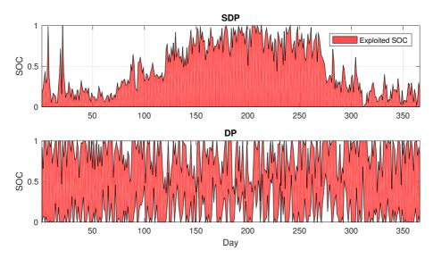
Figure 5.24: Exploited SOC for standard settings without PV under the power based UT.
