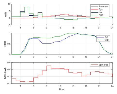
**Figure 5.14:** Wednesday the 22nd of June 2016, standard settings with PV and the power based UT. Upper plot shows  $P_{grid}$  for the basecase, DP and SDP as well as  $P_{PV}$ . Middle plot shows the SOC of the battery. Lower plot shows spot price.
