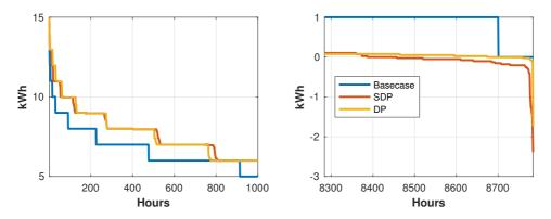
**Figure 5.30:** Duration curves of  $P_{grid}$  for 2016 for load 3 without PV under the energy based UT. Maximum 1000 values and minimum 500 values.
