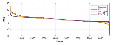
Figure C.3: Duration curves of  $P_{grid}$  for 2016 for load 3 with PV under the power based UT.
