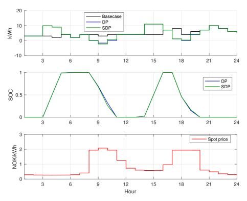
**Figure 5.8:** Thursday the 21st of January 2016, standard settings without PV under the energy based UT. Upper plot shows  $P_{grid}$  for the basecase, DP and SDP. Middle plot shows the SOC of the battery. Lower plot shows spot price.
