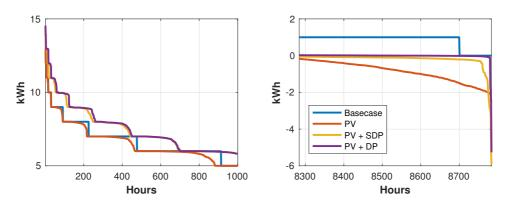
**Figure C.4:** Duration curves of  $P_{grid}$  for 2016 for load 3 with PV under the energy based UT, zoomed in for maximum 1 000 hours and minimum 500 hours.
