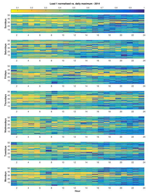
Figure D.2: Normalised load for load 1 in 2014, sorted by days.
