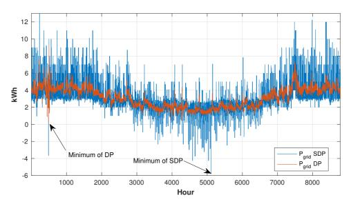
Figure 5.35:  $P_{grid}$  with SDP and DP for 2016 for load 3 without PV.
