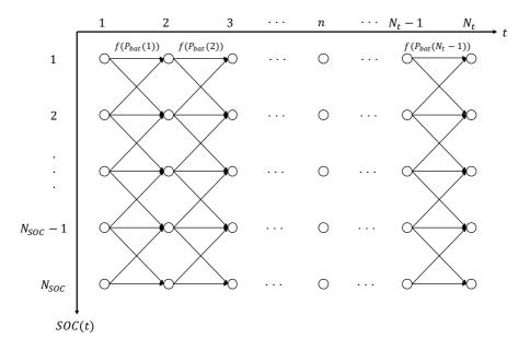
Figure 2.1: Illustration of a DP problem with  $N_t$  time steps and  $N_{SOC}$  states of SOC.
