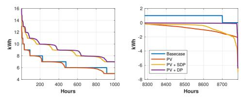
Figure C.5: Duration curves of  $P_{grid}$  for 2016 for load 3 with PV under the time based UT, zoomed in for maximum 1 000 hours and minimum 500 hours.
