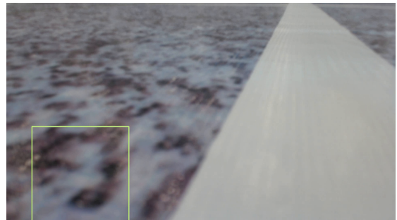
(d) Example of incorrect labeling. The network still finds ghost robots in the floor pattern, but significantly less frequent than SSD300.
