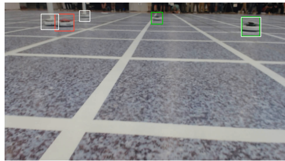
(d) Example of incorrect labeling. Two robots of different colors are detected at almost the same position to the right.
