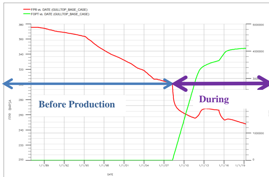
Figure 5: Variation of average reservoir pressure with oil production
