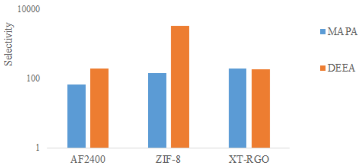
Figure 4.15: CO 2 /amine selectivity in membrane contactor of AF2400/ZIF-8, AF2400/XT-RGO and pure AF2400 at 50°C.
