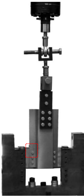
(c) Front of the test rig. Red rectangle shows the location of the DIC mesh (see Fig. 4e).
