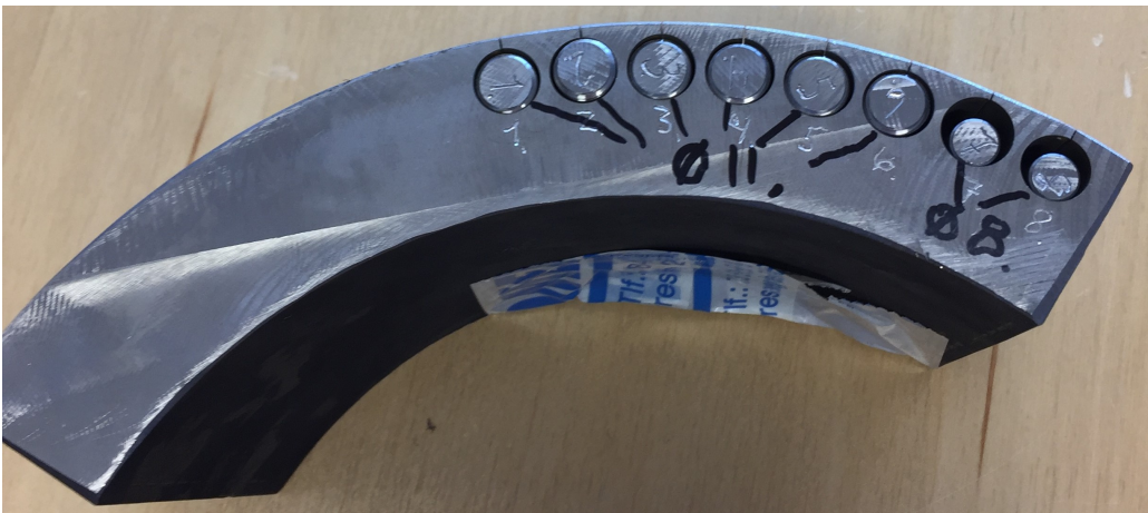
Figure 4: Image of the test specimen location for material E.
