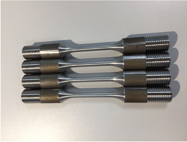
(a) Image of HISC test specimens.
