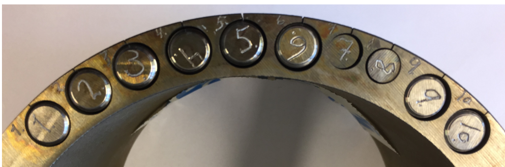
Figure 2: Image of the test specimen location for material C.
