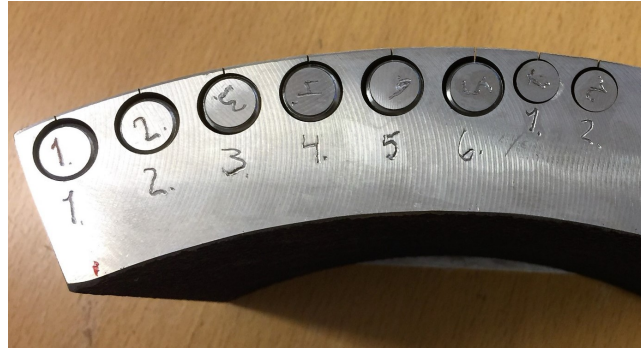
Figure 3.1: Location in test material from which test specimens were cut.
