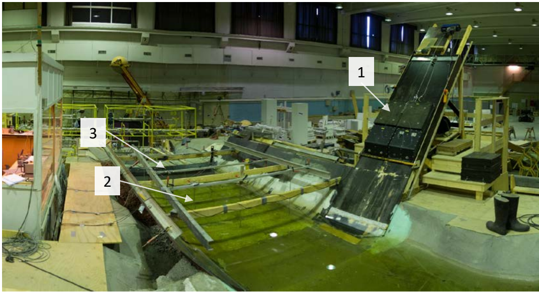
Figure 4.1. Picture of the model with the landslide (1), the reservoir (2) and the overtopped dam (3)
