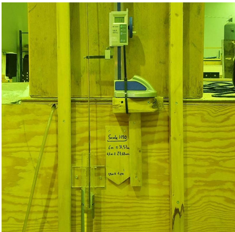
Figure B.1. Piezometer and point gauge used for setting the reservoir level
