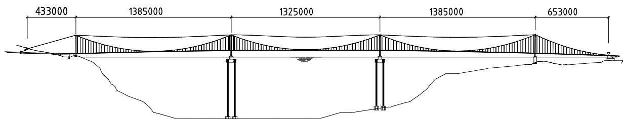
Figure 2.3: General layout of the bridge, (NPRA, 2016j)
