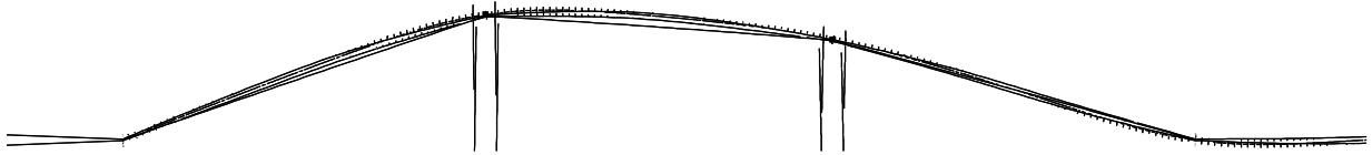
Figure 7.1: First horizontal mode shape from the ABAQUS model viewed from above.
