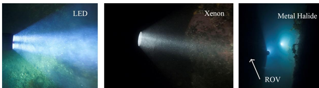
Figure 4.4: LED, XENON (SCUBA), and Metal halide Lamps on ROV. The images are taken from the side of the light source and visualize the light beams (Photos: Geir Johnsen).
