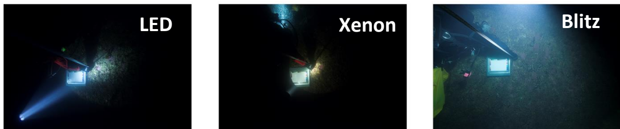
Figure 3.10 – Images taken by SCUBA (Canon) from approximately 1 m illuminated with LED, Xenon and blitz as marked in the upper right corner of each image. The illumination coverage between the three sources was 17 % (LED), 9 % (Xenon) and 80 % (Blitz).
