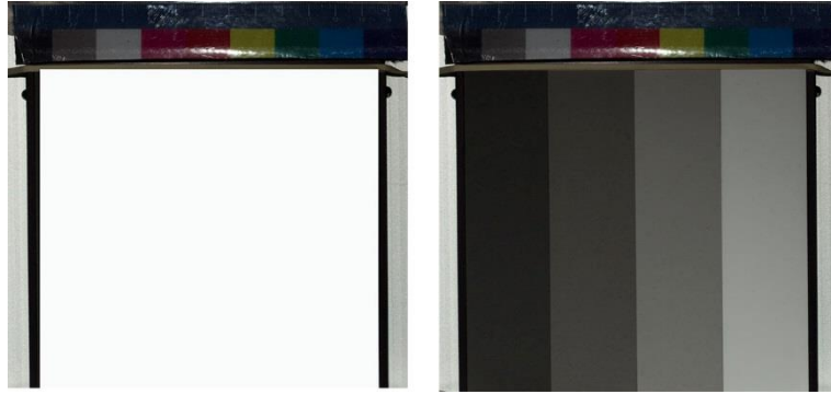
Figure 2.4 – White and greyscale spectral reference plate with colour palette above, picture taken in air from 1.4 m. White balance on camera set to Tungsten and lamp was Halogen (Green Force).
