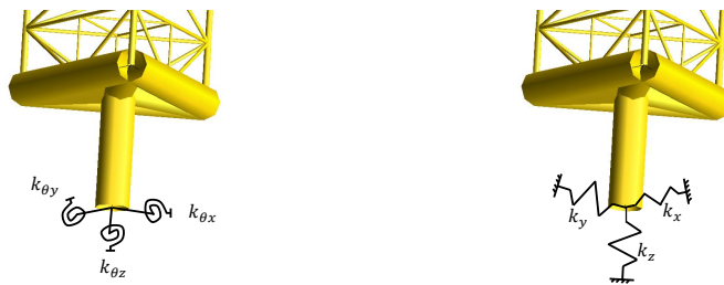
Figure 4.7: Bottom model of one of the legs. Left: rotation springs, Right: Translation springs
