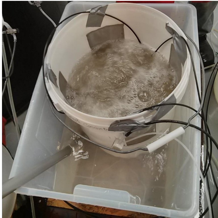
Figure 2.6 Nauplii concentrator consisting of 4 filter frames (40 \mu m mesh size iron sieves) on the side wall and attaching with strong aeration on each frame. Photo: Anh Phan Hung, 2014.
