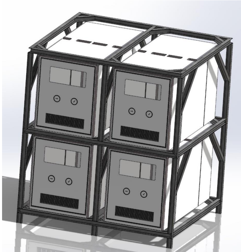
Figure 26 – Initial base frame design with canopy mounted.
