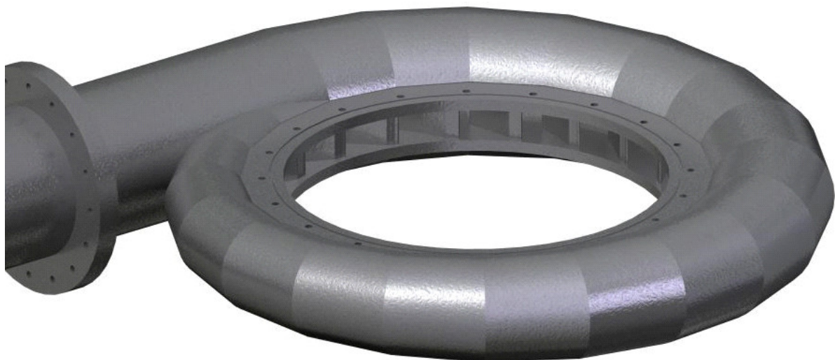
Figure 4-26: TTL Spiral Casing with Stay Ring and Stay Vanes; 3D View
