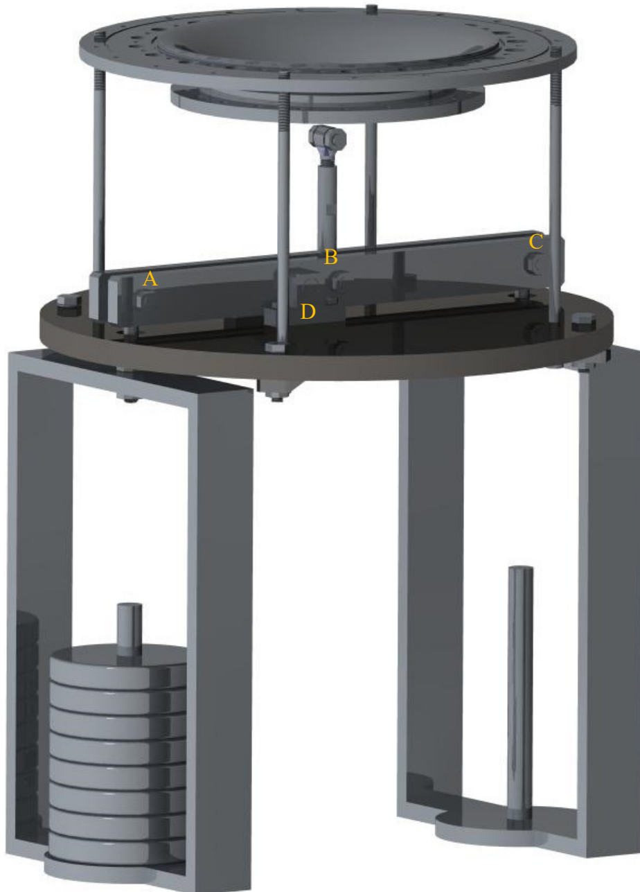
Figure 3-8: Calibration Jig (Weights for Calibration of Upward Axial Force)
