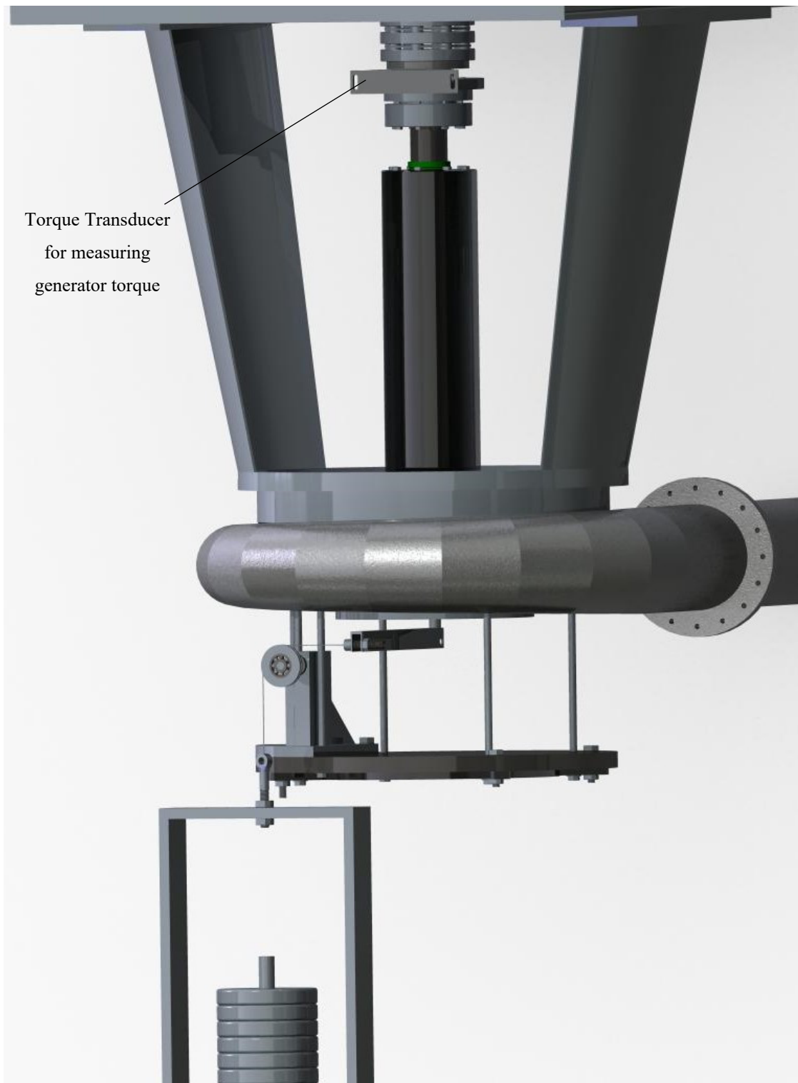
Figure 4-18: TTL Torque Calibration Jig Overview
