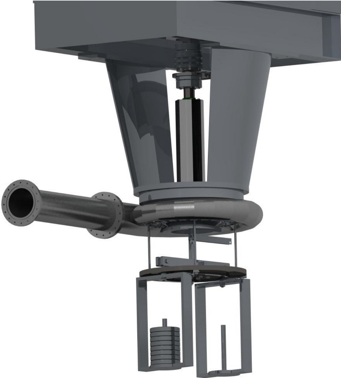
Figure 4-42: TTL Axial Force Calibration; 3D View
