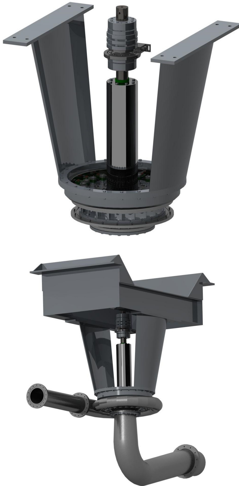
Figure 4-24: TTL Suspension Cone; 3D View
