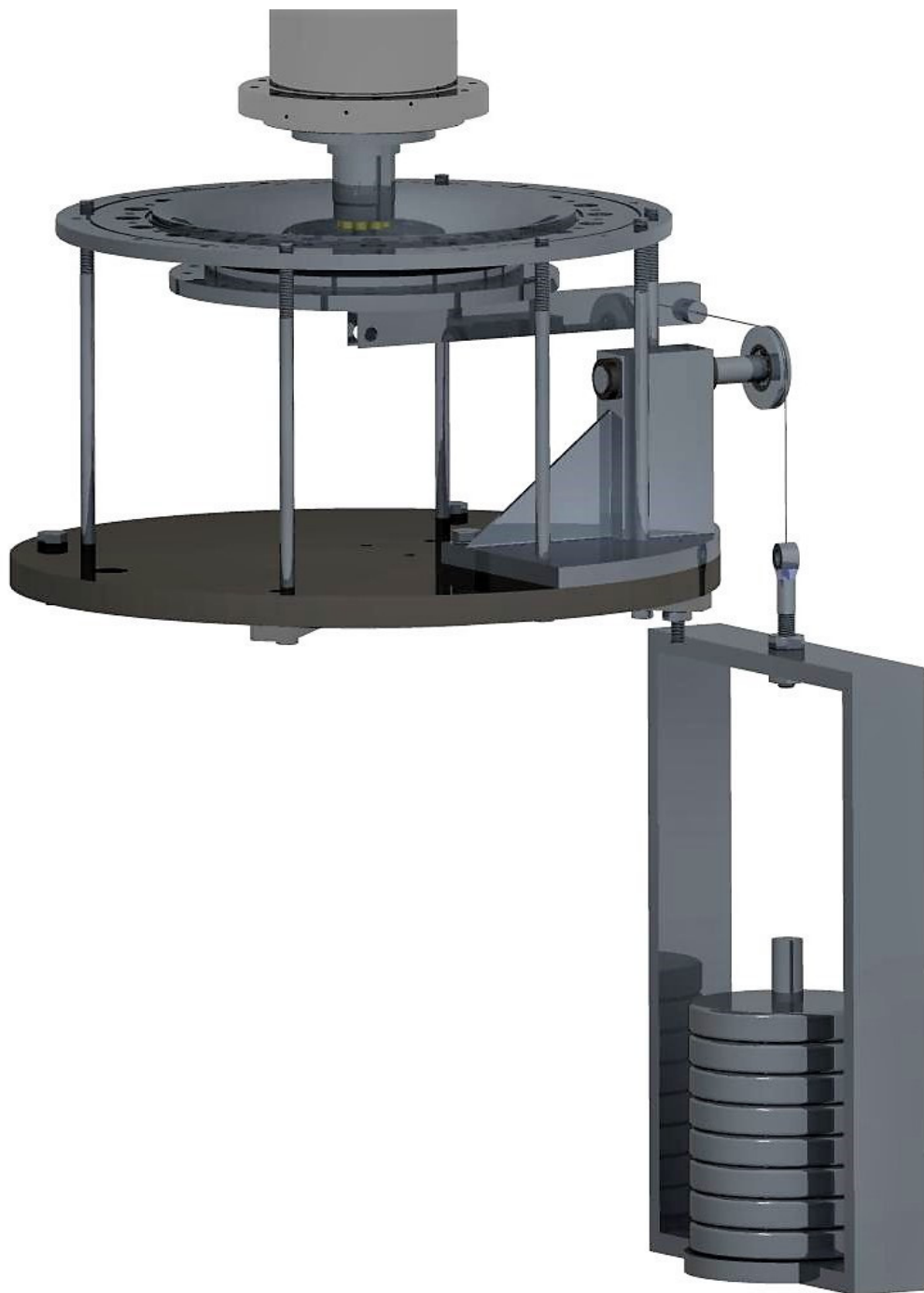
Figure 4-19: TTL Torque Calibration Jig Attached to Bottom Cover
