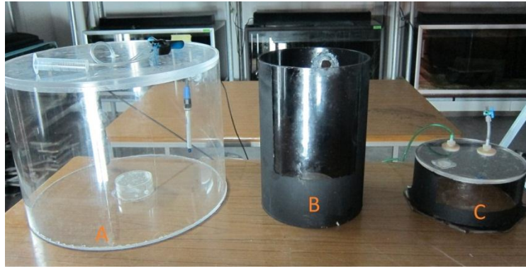
Figure 4a: The three sizes of respiratory chambers used in the experiments with A) snow-trout (50 L), B) group of Red Zebra (12 L) and C) single individuals of Red Zebra (3.7 L). During snow-trout experiments, the chamber wall was covered with black folded plastic bags in similar manner as of chamber B and C.
