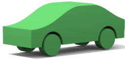
(a) A car formed by taking a rounded union between two cubes, and forming the wheels with cylinders.
